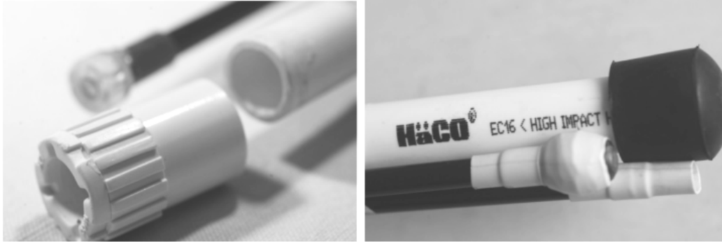
Fig. 6 A sixteen mm diameter PVC tube used for electrical wiring with its end-cap is used as the carbon rod container. Only one end cap is glued. The other end has a removable cap.
