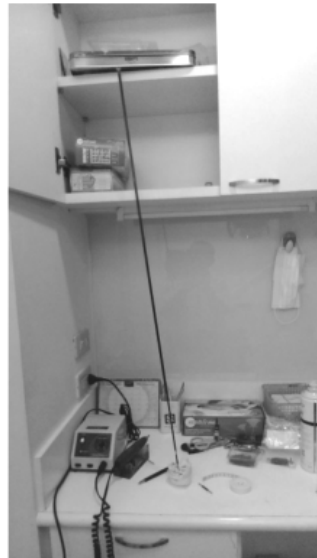
Fig. 2 In confined spaces, a metal biscuit box can replace the glass slab base and the selfie stick. The push pin magnet attaches to the metal box with sufficient force to hold the carbon fiber tube. This technique provides extra working length to the vertical arm, which is useful in certain circumstances.
