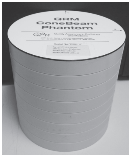
Figure 3 QRM-ConeBeam phantom used for geometric accuracy analysis
