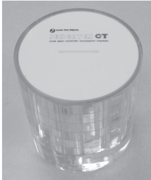
Figure 2 SEDENTEXCT IQ phantom used for technical image quality analysis
