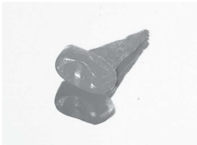
Figure 1: Resin pattern of post and core
